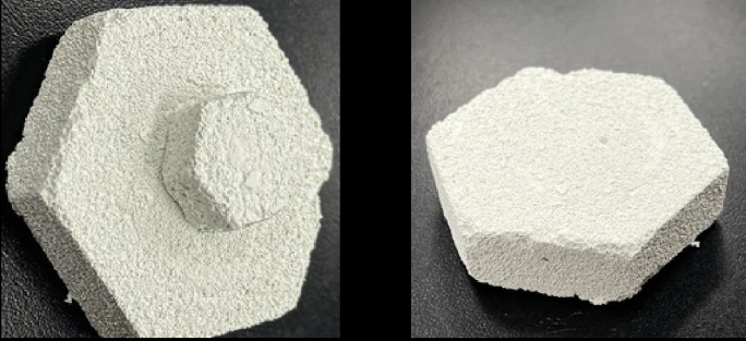
Figure 1 & 2: A hexagonal block of the Novum Coral composite of hydroxyapatite and calcium carbonate
