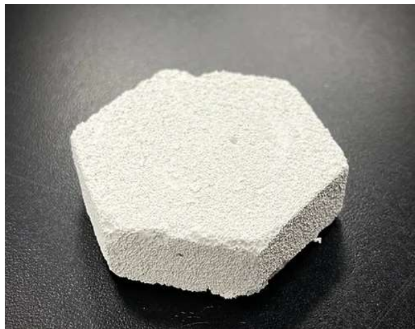
Figure 1: A hexagonal block of the Novum Coral composite of hydroxyapatite and calcium carbonate
